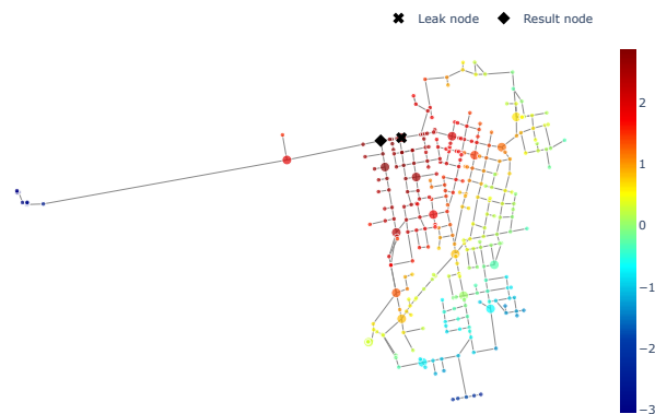
Figure 6: Leak in node J316, 1 a.m.(13 hours from leak start)
